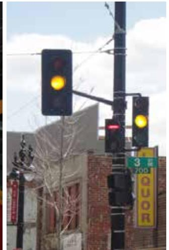
*(L) Streetcar signal indicating it is safe for the streetcar to proceed straight. (R) Streetcar "stop" signal in between regular signals.*
