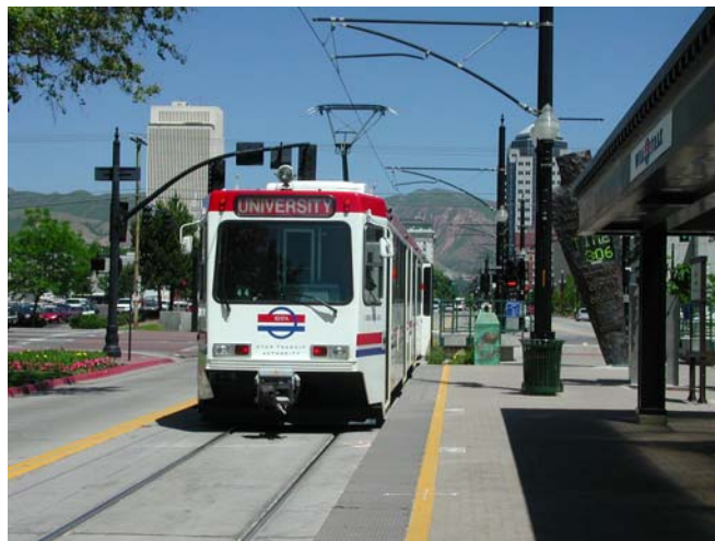
Fig. 1 - Side Cantilevered Support Arms (Salt Lake City, UT)
