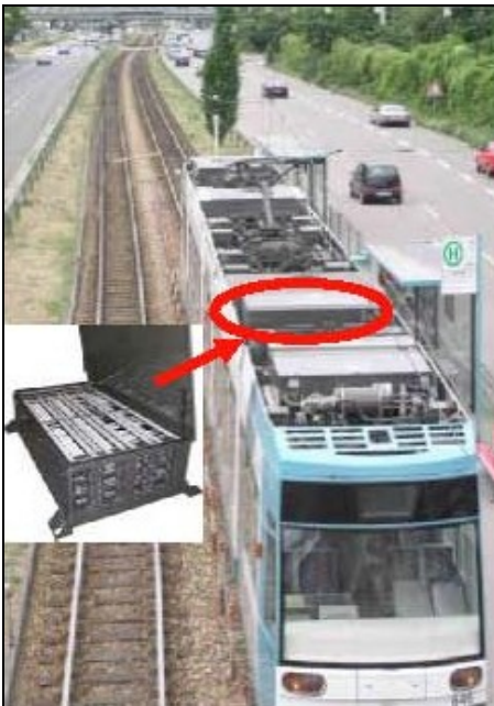
Fig. 22 - Bombardier Mannheim LRV with Ultracapacitor Bank
