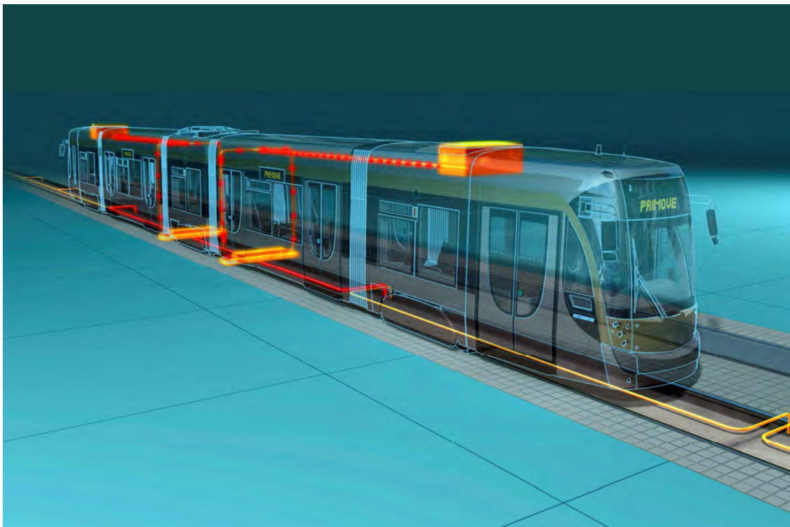
FIGURE 4 Bombardier's PRIMOVE system. a) Technology base. b) Vehicle's diagram. Courtesy of Bombardier.
