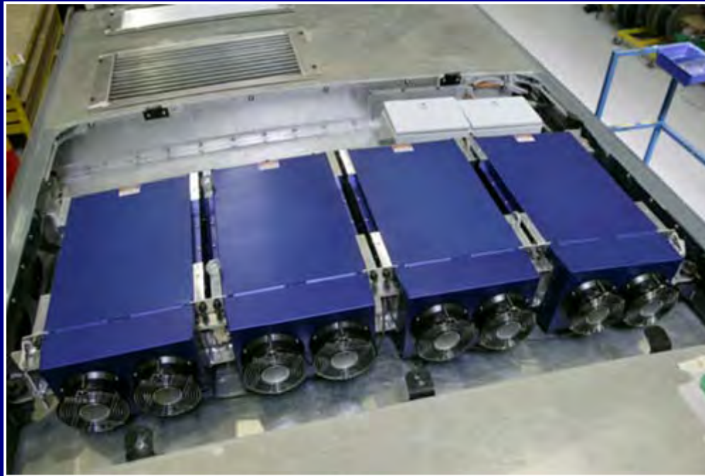
Banks of Supercaps on the roof of a Scania bus.
