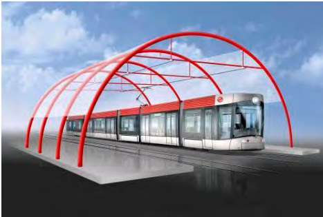
Fig. 6: Recharging station with “overhead busbar”
