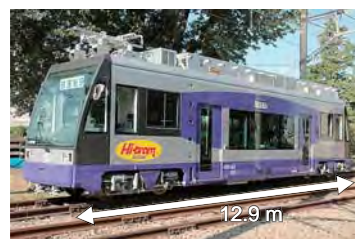
Fig. 3 Contact-wire/battery hybrid LRV
