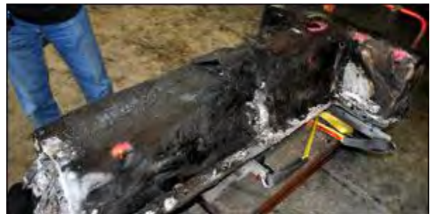
An EV battery damaged in a crash test started a fire that destroyed four vehicles at a test facility in Wisconsin. (Photo: NHSTA)
