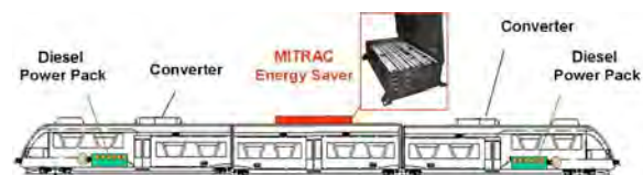
Fig. 12: Principle scheme of a diesel electric vehicle equipped with MITRAC Energy Saver
