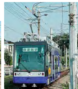
Fig. 4 Quick charging from rigid contact wires
