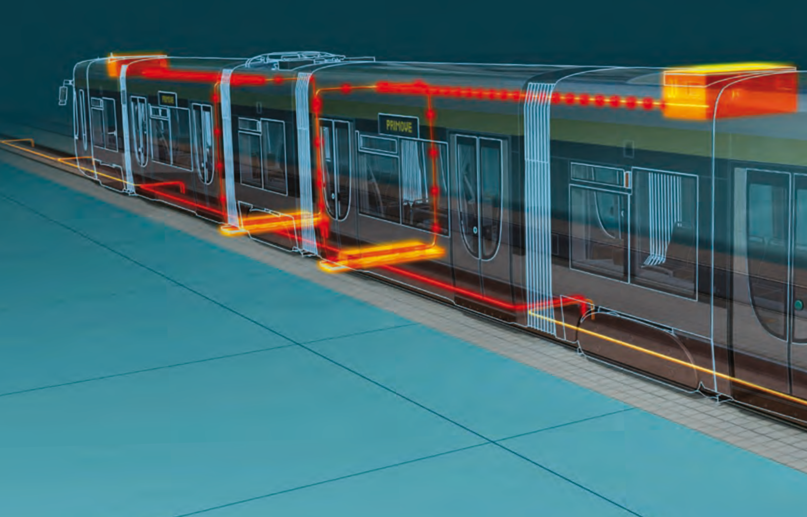
Catenary-free operation – energy flow
