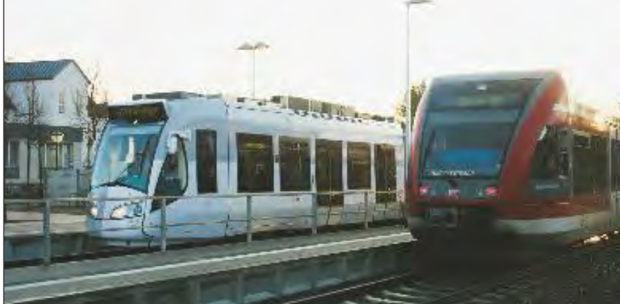
The village of Weimar near Kassel, where light rail and heavy rail share tracks. On the left is a diesel-hybrid tram, on the right is a Stadler GTW DMU of the Kurhessen Bahn. Heribert Menzel
